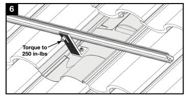
Attach rail to either side of L-Foot with bonding hardware. Ensure L-Foot does not extend above rail. Torque hardware to 250 in-lbs (21 ft-lbs).
