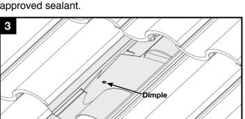
Insert Tile Replacement Flashing, lower onto base and apply pressure over the threaded post until it dimples the flashing.
