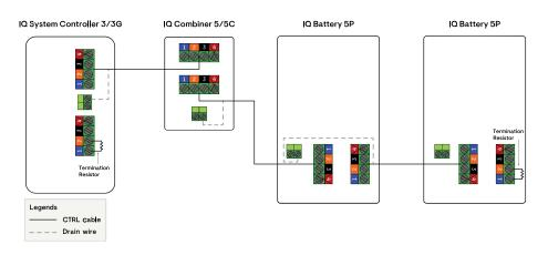
NOTE: The total length of CTRL wiring across the system should not exceed 250 feet to ensure the system operates as per specifications.
