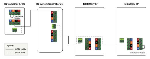
NOTE: The total length of CTRL wiring across the system should not exceed 250 feet to ensure the system operates as per specifications.
