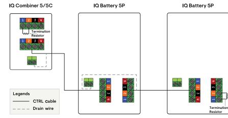
NOTE: The total length of CTRL wiring across the system should not exceed 250 feet to ensure the system operates as per specifications.
