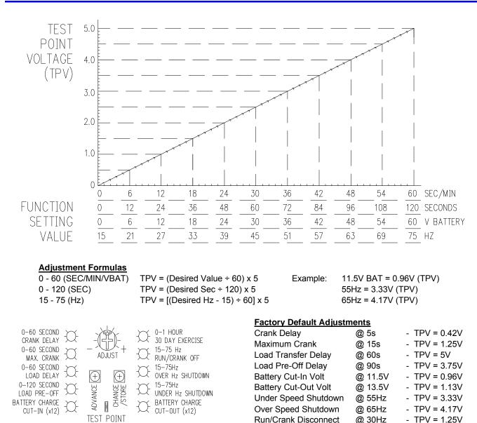
Setting the following adjustments to 0 Volts or 5 Volts on the test point causes the GSCM to operate as follows:
