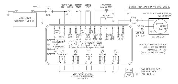
A pressure or level switch starts a direct engine driven pump similar to Application 5. The K5 (load transfer) relay is used to energize the pump unloader valve closing when the engine is running. The unloader valve bleeds off the pump pressure when de-energized. The standard GSCM "out of the box" looks for a minimum 100V AC frequency input signal. Order a special low voltage generator frequency input version for 12V alternator applications. See Sections 3:9 & 4:9.
