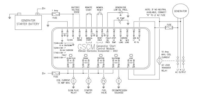
The diesel generator is started by the GSCM in either automatic or manual mode. A field installed relay that will handle the glow plug current is needed if not already installed on the engine. A fuel control solenoid is connected to the K3 (ignition) relay terminals. A decompression solenoid furnished with the generator must be wired to K4 (shutdown) relay to energize on shutdown.
