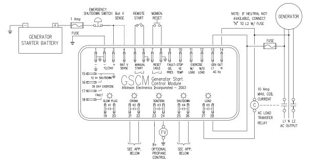
This application matches most high speed or portable generator sets that have an electric starter and some type of starter control. These generators should have the ignition switch left in the 'on' position. The start commands usually come through the GSCM connected to the remote start terminals. The remote start may be either momentary or maintained.
