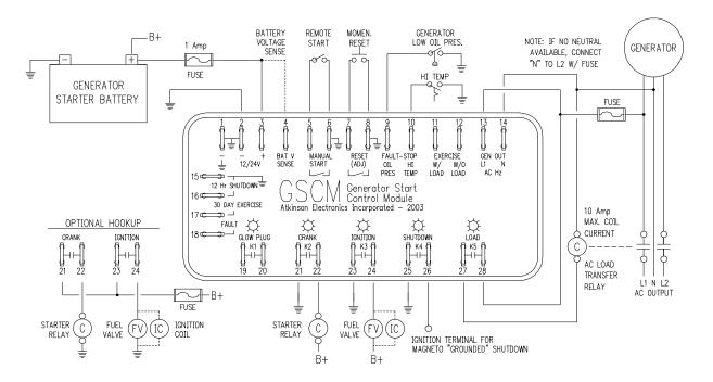
This application matches high speed generators that do not include starter control boxes. Propane generators may be the type that ground the ignition to shutdown or have an automotive type coil ignition. The wiring configurations are shown for both automotive and magneto type with or without fuel valves. High speed (3600 RPM) generators may need the crank disconnect hertz adjustment set to 20Hz or less to avoid over driving the starter.
