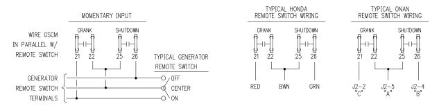
The K2 (crank) relay is used to switch the start input which is looking for a momentary signal. The K2 (crank) relay opens when the generator has reached 30Hz, or half speed. If this setting doesn't allow the start input to remain engaged long enough for the generator to stay on-line, adjust the run disconnect setting to 55Hz (see Section-4 for changing adjustments). The K4 (shutdown) relay provides a momentary "stop" signal until the generator AC Hz has dropped to zero.
