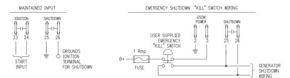
The K3 (ignition) relay provides a continuous run signal for generators requiring a "maintained" start signal. The K4 (shutdown) relay provides a momentary "stop" signal until the generator AC Hz has dropped to zero.
