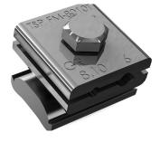
**Ground lug** Use one per module row to ground rail with bare 6 to 10 AWG copper wire. **2 Ground Lugs included.**
