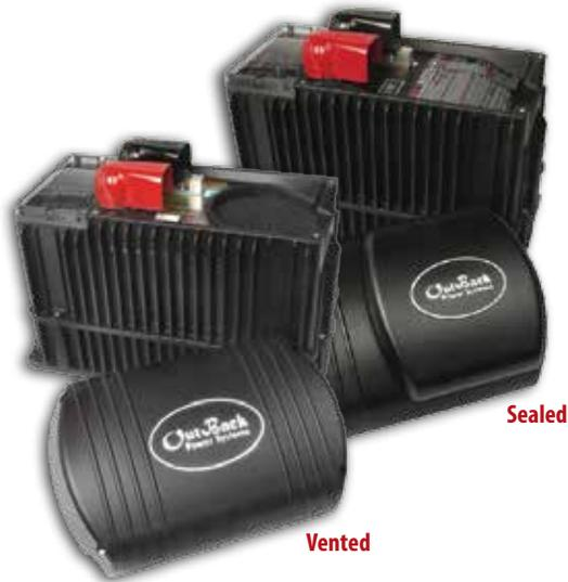
**OutBack Power's true sinewave grid-interactive inverter/chargers incorporate a DC to AC sinewave inverter, battery charger and AC transfer switch housed within a die-cast aluminum chassis.**
