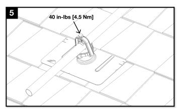
Adjust top bolt so saddle is snug on the conduit. Tighten bolt on top of saddle to 40 in-lb [4.5 Nm].
