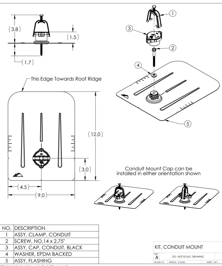
$<sup>^{\</sup>star}$  Bill of materials shown is for a single Conduit Mount assembly.
