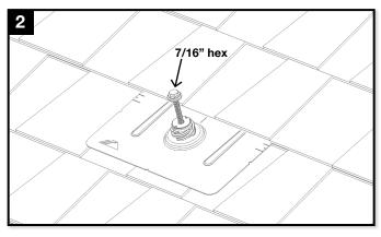
Fill hole in dock with roofing manufacturer's approved sealant. Insert screw with bonded washer through hole. Tighten screw until fully seated.
