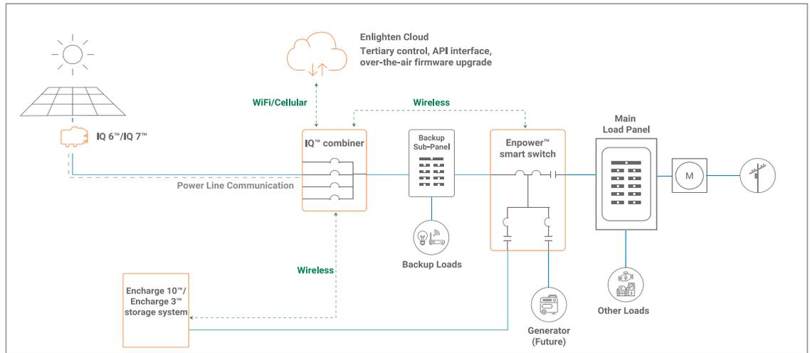
**Self consumption, no Enpower smart switch.** The preferred configuration when adding battery storage and PV for self-consumption in a grid-tied application with no option for backup during outages. PV and Encharge will not operate when the grid is unavailable.
