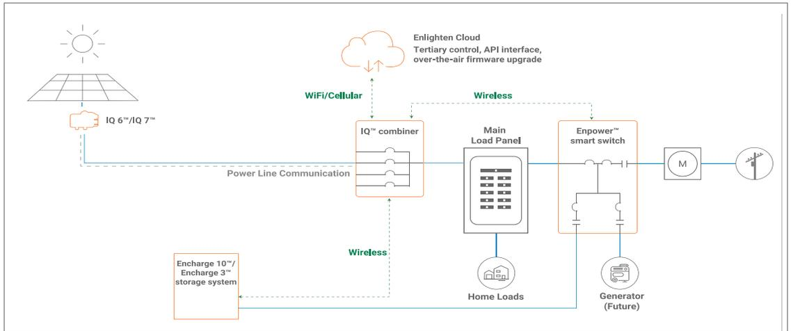
**Partial home backup with main load panel as service entrance and PV combiner connected to Enpower.** When PV circuits breaker size is less than 80A, this is the preferred configuration for partial home backup with sub-panel.
