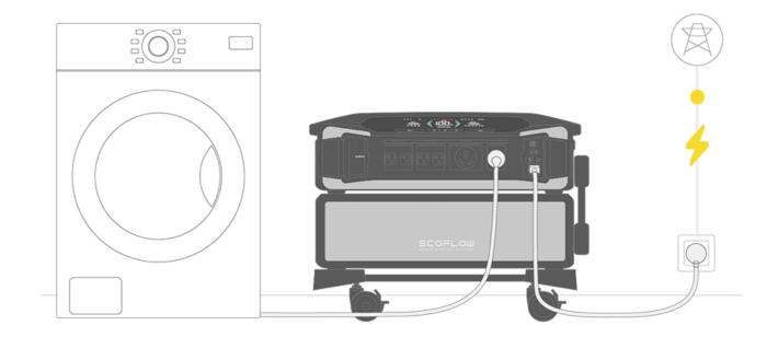
X-Fusion is an advanced technology that ensures all AC output sockets provide optimal output when the product is in bypass mode (when you recharge and discharge the device simultaneously, the device enables bypass mode automatically), in terms of wattage and amp. In the fast charging mode, the output will always be 7.2kW no matter how much the input is.
