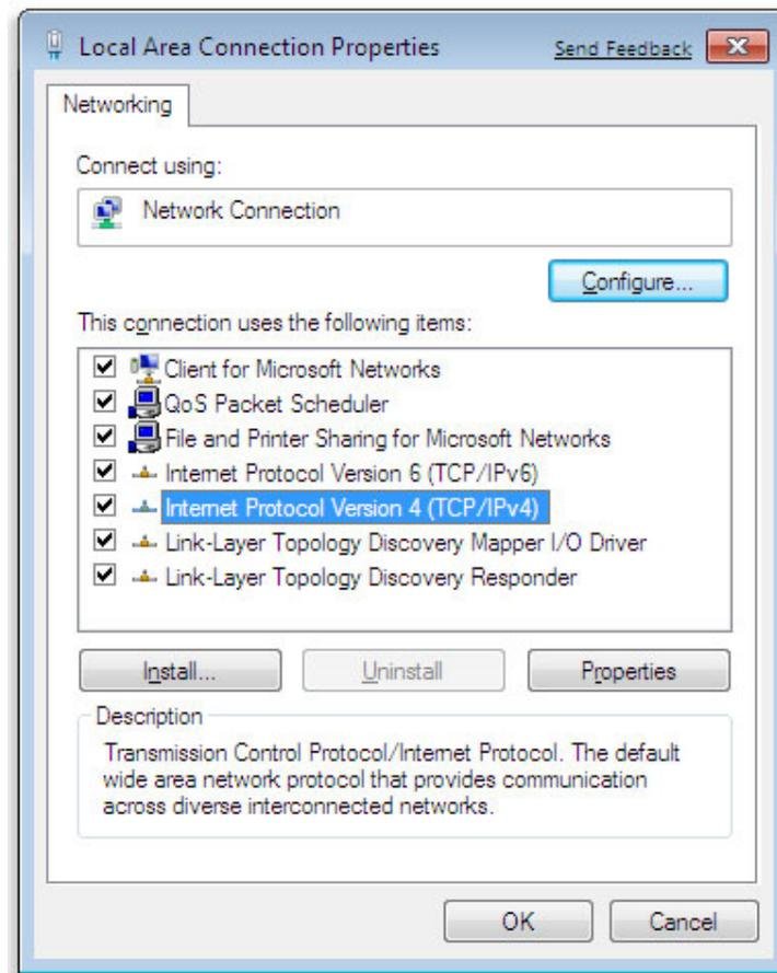
4. In the properties dialog box, click **Use the following IP address:** to configure your computer for Static TCP/IP. Enter an **IP address** (i.e. 192.168.1.10), the **subnet mask** of the ENH202, and the **default gateway** which is the ENH202's IP address, 192.168.1.1. Note: the subnet mask must match that of the ENH202 and the IP address must be on that subnet.
