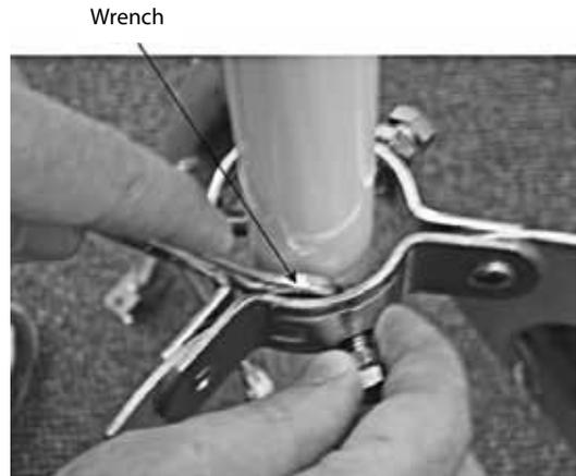
Using a 5" wrench secure the tripod.
