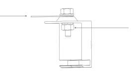
Then tighten the bolt using the toothed nut.
