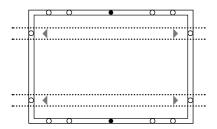
Maximum Load: Uplift load ≤ 2400 Pa Downforce load ≤ 2400 Pa Compatible module type: CS6A-xxxP, CS6A-xxxM, CS6P-xxxP, CS6P-xxxM and CS6A-xxxMS
