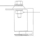
Then tighten the bolt using the toothed nut.
