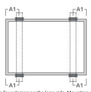
Use four clamps on the long side. Mounting rails run perpendicularly to the long side frame.
