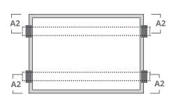
Use four clamps on the short side. Mounting rails run parallel to the long side frame.
