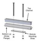
End clamps are attached to the module at the end of each array and in the middle next to the gear drive. Four end clamps are used for each row of modules. End clamps are at least 22" long and have four attachment holes. End clamps also include a spacer plate (fabricated for each specific module) that must be inserted in the clamp on the outside of the clamp (opposite the end module) to maintain a balanced force with the end module.
