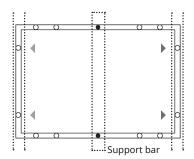
Maximum Load: Uplift load  $\leq$  2400 Pa Downforce load  $\leq$  5400 Pa Compatible module type: CS6A-xxxP, CS6A-xxxM, CS6PxxxP and CS6P-xxxM
