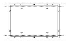
Maximum Load: Uplift load ≤ 2400 Pa Downforce load ≤4000 Pa Compatible module type: CS6A-xxxP, CS6A-xxxM, CS6VxxxP, CS6V-xxxM, CS6P-xxxP, CS6P-xxxM, CS6K-xxxP, CS6K-xxxM, CS6X-xxxP and CS6X-xxxM
