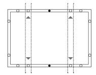
Maximum Load: Uplift load ≤ 2400 Pa Downforce load ≤ 5400 Pa Compatible module type: CS6A-xxxP, CS6A-xxxM, CS6V-xxxP, CS6V-xxxM, CS6P-xxxP, CS6P-xxxM, CS6K-xxxP, CS6K-xxxM, CS6X-xxxP CS6X-xxxM, CS6K-xxxMS, CS6V-xxxMS and CS6A-xxxMS Bolting on short frame side using four standard mounting holes. An additional support bar should be placed below the module. Mounting rails should run parallel to the short frame side
