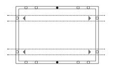
Maximum Load: Uplift load  $\leq$  2400 Pa Downforce load  $\leq$  2400 Pa Compatible module type: CS6A-xxxP, CS6A-xxxM, CS6P-xxxP, CS6P-xxxM and CS6A-MS
