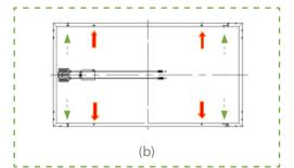
Remark: As for above diagram, the solid red arrows indicate primary bolt positions; dashed blue arrows indicate positions where bolts can be added for additional support.
