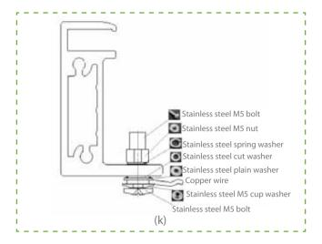
Grounding the aluminum frame with copper wire
