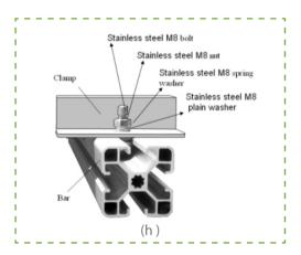
6. Especially for Fig. (d) mounting method, slide bolts through groove on the supporting bars next to the locations where the 4 clamps are to be fastened. The module may be clamped only in the permitted clamping are as on the long edge of the frame. For exact locations on the frame refer to Fig. (i) in conjunction with table 1 below.
