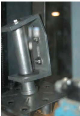
Figure 6 - Pull test failure- two bolts
