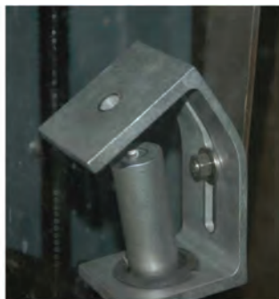
Figure 5 - Pull test failure- one bolt
