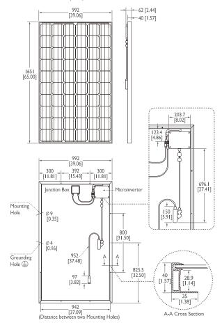
BenQ Solar AC Unison is a new breakthrough in solar photovoltaic (PV) technology. BenQ Solar combines its premium PV module with reliable microinverter technology to maximize PV benefits for installers and end users.
