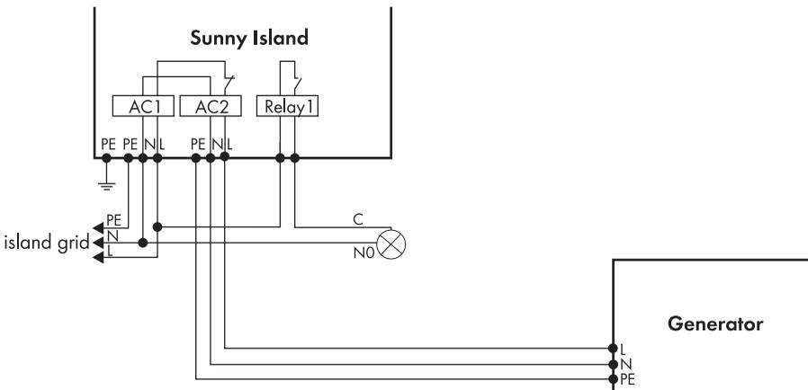
The generator is also always switched off manually. The Sunny Island then automatically switches to operation without generator.
