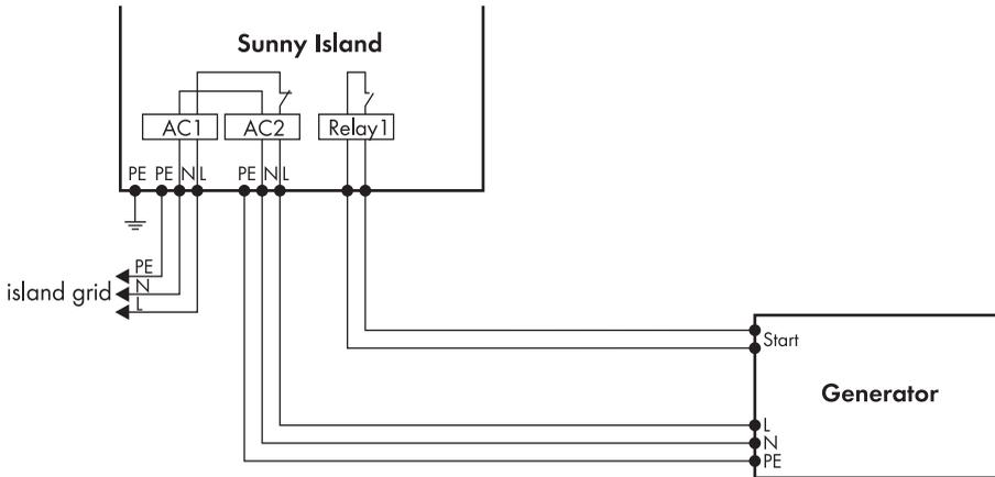
If the generator is started manually in this operating mode, the Sunny Island detects the running generator and connects once the warm-up time has expired. If the generator is externally stopped, this is detected, the generator is disconnected and the stand-alone grid is continued to be supplied.
