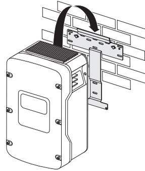
6. Screw the Sunny Island to the wall mounting bracket on both sides using the screws (M6x10) provided. Tighten the screws clockwise.
