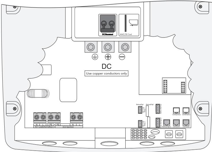
Use conduits to install the cables on the DC side and on the AC side on the Sunny Island. Conduits ensure the dust-tight and water-tight mounting of the cables on the enclosure and also serve as a strain relief of the cables at the connection. Close all unused openings in the enclosure using the appropriate filler plugs.
