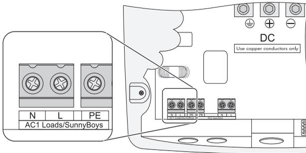
5. Insert PE into the terminal labeled "AC1 Loads/Sunny Boys" and tighten the fastening screw with a torque of 22 in-lbs. (2.5 Nm). Use a torque wrench with flat-blade screwdriver bit SZS 1.0 x 6.5.
