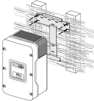
If two or more Sunny Island inverters have to be installed, mount the inverters on two studs each in order to get better cooling. Make sure that the wall where you intend to install the Sunny Island is vertical and can carry the weight of the Sunny Island (139 lbs, 63 kg) on a long-term basis.
