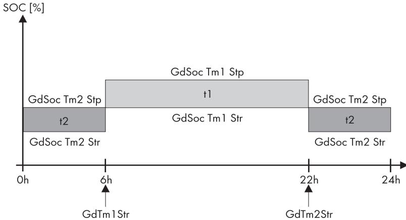
The Sunny Island connects to the grid, when the state of charge of its batteries lies within the limits determined by the following parameters:
