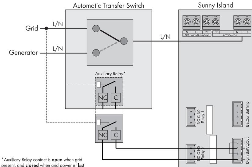
In order to switch the signal circuit via the DigIn input, a single pole break contact or a single pole auxiliary relay with a 120 V coil is necessary. If there is no auxiliary relay present in the ATS, you must install an external contactor with a 120 V or 240 V coil. The coil is supplied with voltage via the utility grid.
