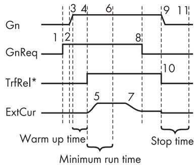
**Generator Interface "234.07 GnSrtMod" = Autostart; Request Via Sunny Island**
