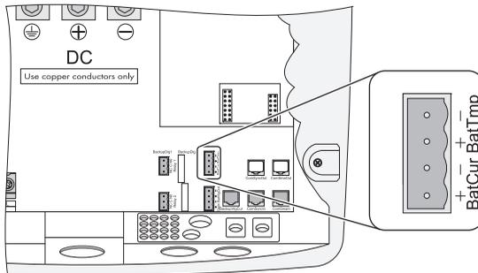
3. Connect the insulated conductors correspondingly to the "BatTmp" terminal of the 4-pole terminal included in the delivery.
