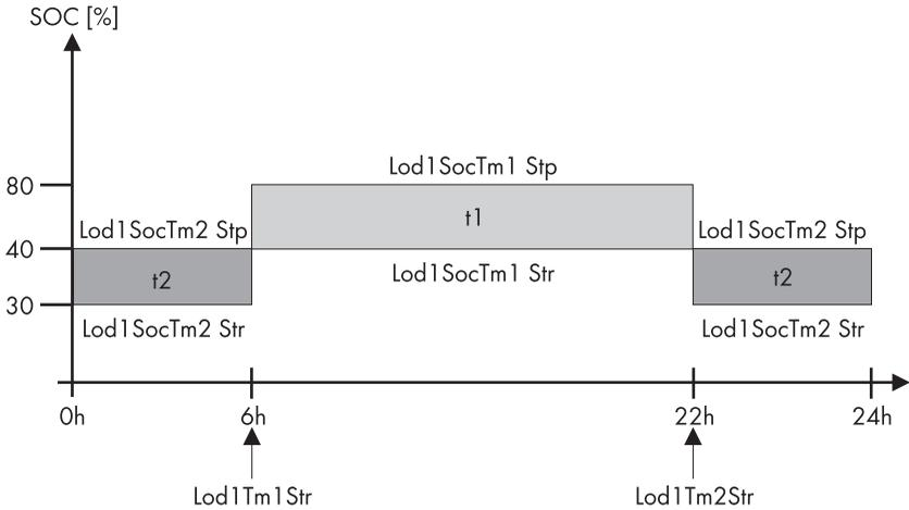
The figure shows an example of the settings if the one-step load shedding function at night is to be avoided as much as possible. From 6:00 a.m. to 10:00 p.m. the load shedding is activated for a state of charge (SOC) of 40%, at nighttime (from 10:00 p.m. to 6:00 a.m.), however, the state of charge of the battery is allowed to go down to 30% before the load-shedding contactor is activated.
