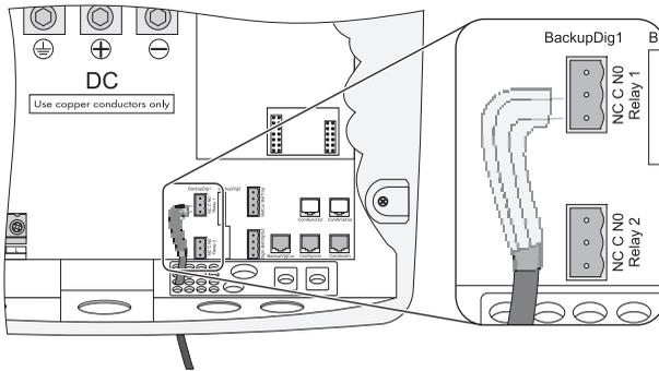
4. Connect the conductors to the supplied three-pole terminals. The pins have the following meaning:
