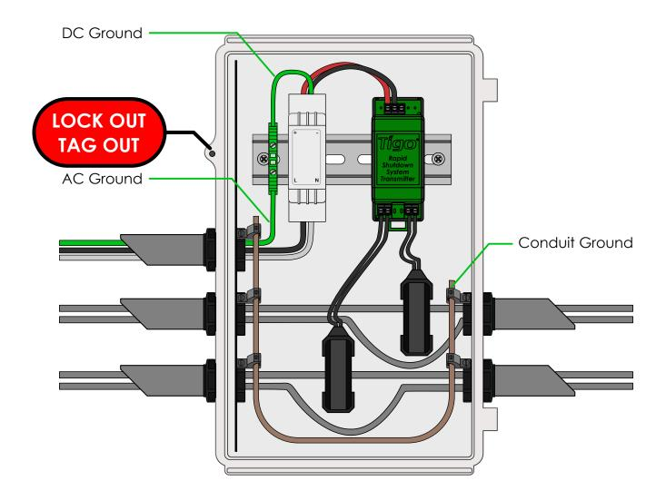
Note: Install TS4-F <u>before</u> powering on RSS Transmitter
