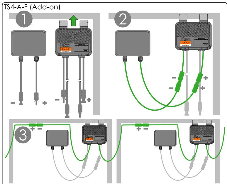
Note: When installing TS4-A-F, connect the input cables to the PV module before connecting the TS4-A-F output cables in series.
