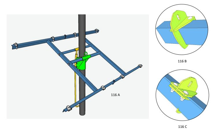
116: Plan the layout of your rails according to your module width. Install the Beam Clamps on the I-beam using the 3/8" x  $1\,1/4$ " carriage bolts and 3/8" flange nuts.
