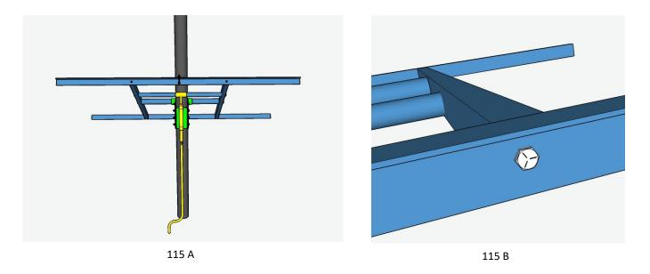
115: Standing on the North Side of the array with the Tube to Angle bolts started but not tightened, sight the Angle pieces to ensure they are parallel. If not, twist the array until they are then tighten the bolts between the Rectangular Tubes and the Angle.
