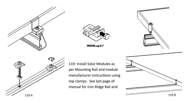
119: Install Solar Modules as per Mounting Rail and module manufacturer instructions using top clamps. See last page of manual for Iron Ridge Rail and Clamp instructions.
