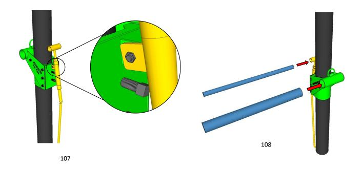
107: Attach the Screw Adjuster to the tab on the Back Plate with the  $1/2" \times 1 \ 1/2"$  Bolt, two 1/2" flat washers and 1/2" Nylock Nut.
