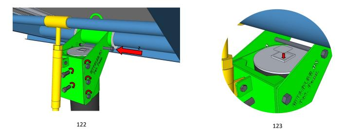
122: Insert the last 3/4" x 9" bolt over the top of the pole with the 3/4" flat washers and 3/4" nut. Securely tighten the tension bolts in the back mounting plate to 200 ft-lb and all 3 bolts through the U Bracket Assembly and the back mounting plate.
