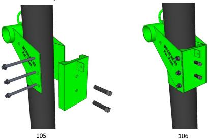
105: While holding the U-Bracket around the pole, insert 3 of the 3/4" x 9" bolts through the holes in the back of the U-bracket and through the holes on the Back Plate with 3/4" flat washers on both sides and 3/4" nuts.
