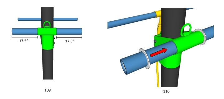
109: Center pipes in sleeves. There should be approximately 17.5" of the 2.5" pipe on either side of the sleeve.
