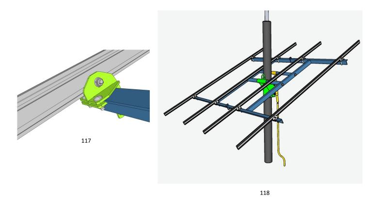
117: Install the Mounting Rail into the beam clamps slot as per Mounting Rail instructions. Use 3/8" x 1" stainless steel bolts and 3/8" serrated flange nuts. Tighten beam clamps once the rails are in position for modules.
