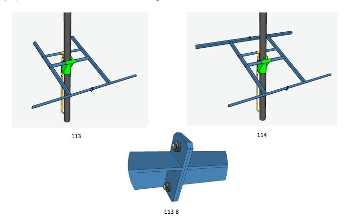
113: Install the first two 3x2 Angle sections to the 2x3 Tube using the  $1/2" \times 1 \times 1/2"$  bolts, flat washers and split washers. Use the  $1/2" \times 1 \times 1/4"$  bolts and 1/2" flange nuts to splice the two angle sections together.
