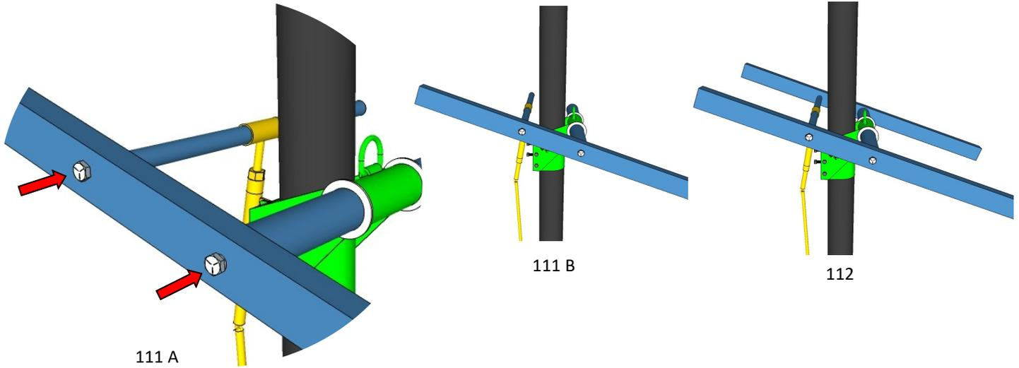
111: Ensure that the MT Solar lettering is upright, and attach one of the 2x3" rectangular tubes to the 2.5" pipe and 2" pipe using the 1/2" x 3 1/2" bolts with 1/2" flat washers and split washers.
