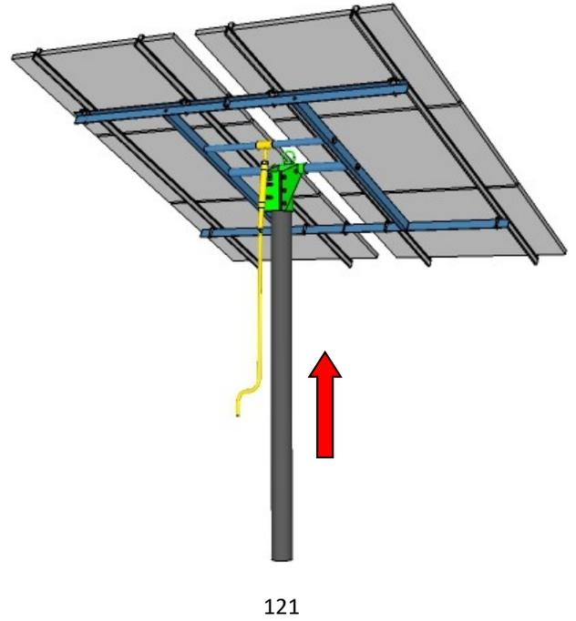
120: Once module installation is complete, raise and or tilt the array to facilitate module wiring and wire management as needed.
