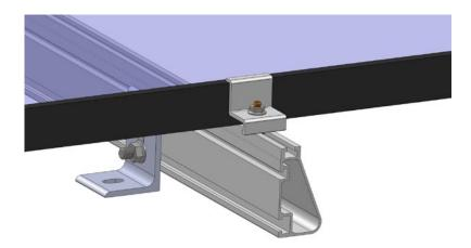
**E.** Working from the opposite side of the PV module. Assemble the mid clamps by putting a clamp on the bolt, followed by the flange nut.
