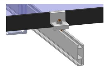
**E.** Working from the opposite side of the PV module. Assemble the mid clamps by putting a clamp on the bolt, followed by the flange nut.
