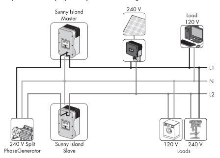
Generally the internal transfer relays of the slaves close only if the internal relay of the master is closed.
