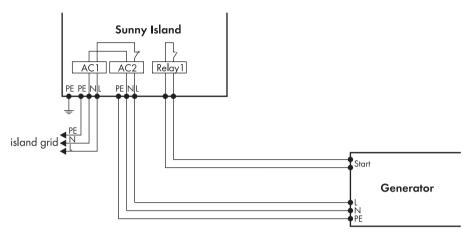
If the generator is started manually in this operating mode, the Sunny Island detects the running generator and connects once the warm-up time has expired. If the generator is externally stopped, this is detected, the generator is disconnected and the stand-alone grid is continued to be supplied.
