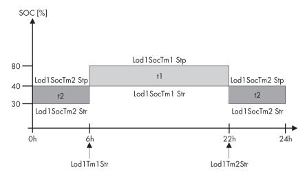
The figure shows an example of the settings if the one-step load shedding function at night is to be avoided as much as possible. From 6:00 a.m. to 10:00 p.m. the load shedding is activated for a state of charge (SOC) of 40%, at nighttime (from 10:00 p.m. to 6:00 a.m.), however, the state of charge of the battery is allowed to go down to 30% before the load-shedding contactor is activated.
