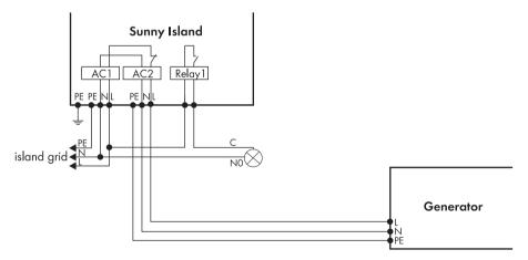
The generator is also always switched off manually. The Sunny Island then automatically switches to operation without generator.
