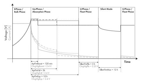
The I stands for the constant current phase (I phase). In this phase, the charging is limited by the maximum defined battery current (parameter "222.01 BatChrgCurMax"), the nominal generator current (parameter "234.03 GnCurNom"), the nominal grid current
