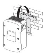
6. Screw the Sunny Island to the wall mounting bracket on both sides using the screws (M6x10) provided. Tighten the screws clockwise.
