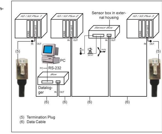
Example of System Component Networking on SolarNet
