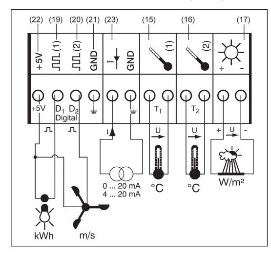
The following describes in detail each measurement signal input in the connection area. Fronius also offers ready-made sensors for measuring ambient temperature, module temperature, irradiance, wind speed and energy.
