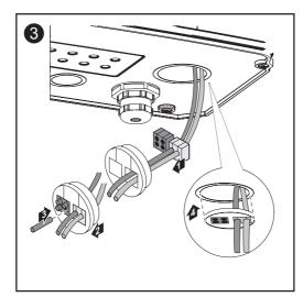
Square sealing inserts are part of the plug-in card scope of delivery.
