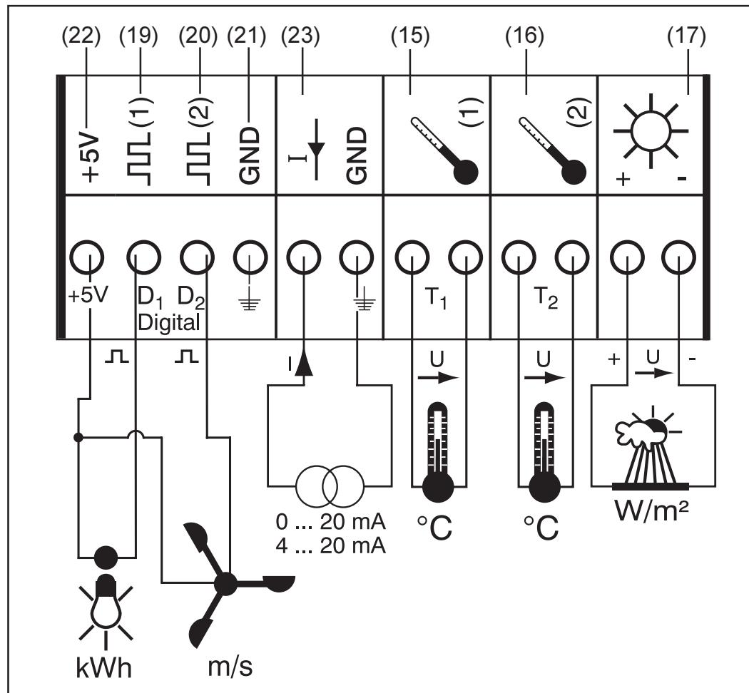
The following describes in detail each measurement signal input in the connection area. Fronius also offers ready-made sensors for measuring ambient temperature, module temperature, irradiance, wind speed and energy.
