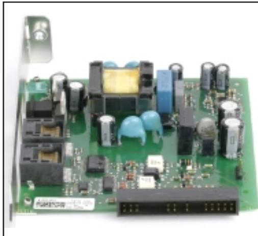
Com cards provide the data link from the Fronius IG or Fronius IG Plus to the SolarNet and to the associated DATCOM components. For this reason, Com cards are only available as plug-in cards. One Com card is required for each Fronius IG and Fronius IG Plus.
