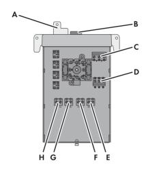
Figure 12: Connection areas of the DC Disconnect
