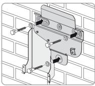
For mounting on a stud or post in a drywall construction, use the two holes at the center.
