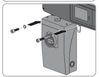
Feed the inverter DC cable through the rubber grommet on the upper side of the DC Disconnect.
