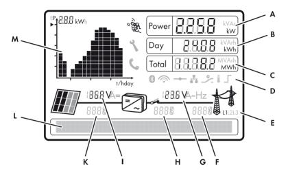
Figure 6: Display layout (example)
