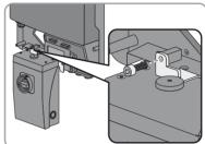
Attach the DC Disconnect to the bracket using the M5x8 screws and conical spring washers included in the delivery and an Allen key (AF 4) (torque: 44in-lbs. (5 Nm)).
