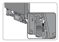
12. Secure the conical spring washer, the grounding cable of the SPS module and the clamping bracket using the cheese-head screw (torque 53 in-lbs. (6 Nm)). The teeth of the conical spring washer must face the clamping bracket.
