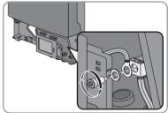
If the display is raised, lower the display and tighten the display screw by hand.
