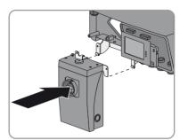
7. Attach the DC Disconnect to the ground connection on the inverter using the grounding bracket. Use the M6x8 screw included in the delivery, the corresponding conical spring washer and an Allen key (AF 5) (torque: 53 in-lbs. (6 Nm)). When doing so, ensure that the holes in the lateral brackets of the DC Disconnect are flush with the holes in the retainer.
