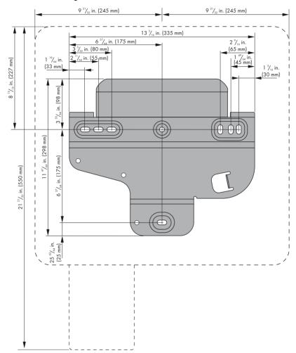
Figure 7: Wall mounting bracket dimensions
