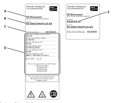
Figure 5: Layout of the type label
