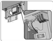
Ensure that no voltage is present between L1 and the equipment grounding conductor.
