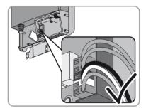
Ensure that the grounding cable of the module is connected to the ground connection in the inverter.
