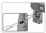
Remove the varistor from the connecting terminal plate.
