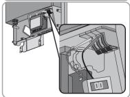
Ensure that no voltage is present between L2 and the equipment grounding conductor.
