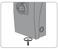
Snap out the required number of knockouts on the desired side of the DC Disconnect for the installation of the conduit fittings (diameter <sup>1</sup>/<sub>2</sub> in., <sup>3</sup>/<sub>4</sub> in. or 1 in.).
