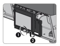
5. Push both detents of the fan casing towards the fan and remove the fan along with the fan casing.
