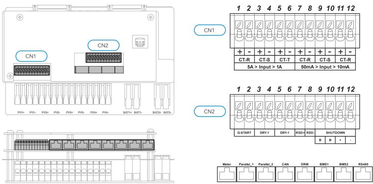
Inverter pinouts for sensors and accessories
