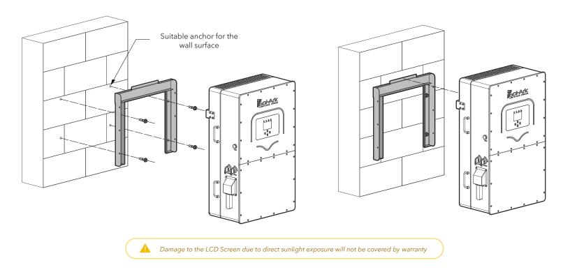
G. Mount the inverter in the optimal orientation as shown below.
