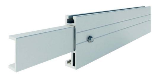
Light Rail Splice bars are structural elements that may be used to join two or more of the IronRidge Light Rails together to create a single, longer rail. Although the splice is structural, the installer must note that the joint will not be as strong as the rail itself.
