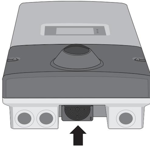
If the fan guards are dirty with loose dust, then you can clean them with a vacuum cleaner. Hold the pipe of the vacuum cleaner below the fan of the inverter (see Figure). If you are unable to clean the fan properly, contact your installer who will dismantle the fan in order to clean it.
