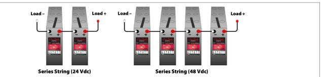
Batteries are placed in series (negative to positive) for additive voltages. Batteries in series are known as a "string". A string of two EnergyCell batteries has a nominal voltage of 24 Vdc and can be used for 24-volt loads. A string of four has a nominal voltage of 48 Vdc. Other voltages are possible. However, batteries in series do not have additive amp-hours. A single string of any voltage (as shown above) has the same amp-hours as a single battery.
