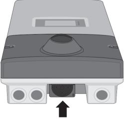
If the fan guards are dirty with loose dust, then you can clean them with a vacuum cleaner. Hold the pipe of the vacuum cleaner below the fan of the inverter (see Figure). If you are unable to clean the fan properly, contact your installer who will dismantle the fan in order to clean it.
