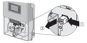
4. Pull the handle of the fan bracket carefully downwards, until the fan bracket is pulled out of its guide rail.
