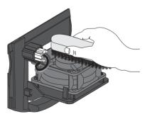
6. Insert the fan and the fan bracket into the guide rail and push upwards.
