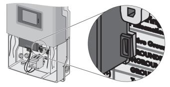
☑ The lug of the Quick module is flush with the lug of the bracket.
