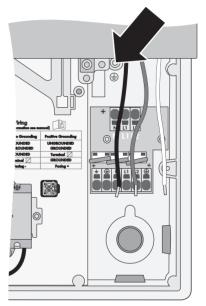
☑ The SMA DC-Disconnect is connected to the Sunny Boy via an electric conductive connection.
