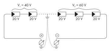
The ground fault is between the second and third module in this case.
