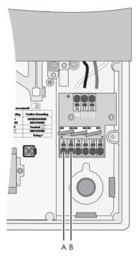
☑ Verify that all connections are correctly wired and properly torqued. Pull the cables in order to make sure that they are sufficiently fixed. The Sunny Boy is connected on the DC side ready to ground the PV plant positively.
