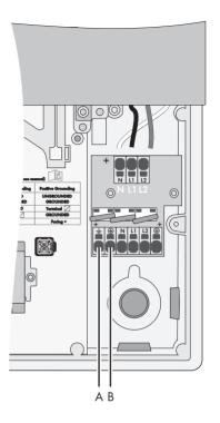
☑ The Sunny Boy is connected on the DC side ready to ground the PV plant negatively.
