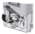
8. Push the Quick Module carefully upwards to the stopper.
