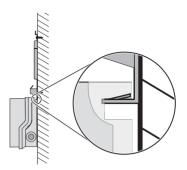
$\blacksquare$  The SMA DC-Disconnect is mounted onto the wall mounting bracket.
