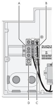
The cables of the PV plant are removed from the DC side of the SMA DC-Disconnect. N
