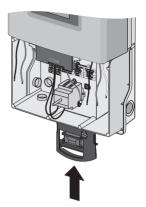
Plug the fan plug into the socket. A click sound can be heard by propper connection. Pull the fan plug slightly to ensure proper connection.
