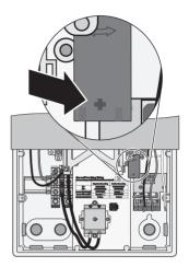
☑ The SMA Plug-in Grounding fuse is changed.
