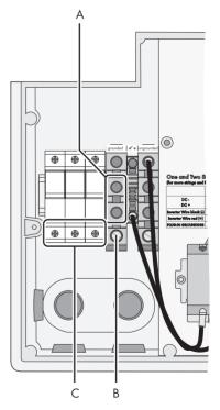
The cables of the PV plant are removed from the DC side of the SMA DC-Disconnect. ☑
