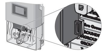
☑ The lug of the Quick module is flush with the lug of the bracket.
