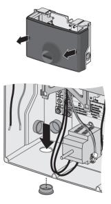
☑ Cable conduits on the DC side are installed and the cables of the PV strings are lead into the Sunny Boy.
