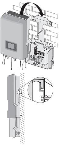
☑ The Sunny Boy is mounted onto the wall mounting bracket.
