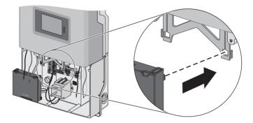
3. Push the Quick Module carefully upwards to the stopper.
