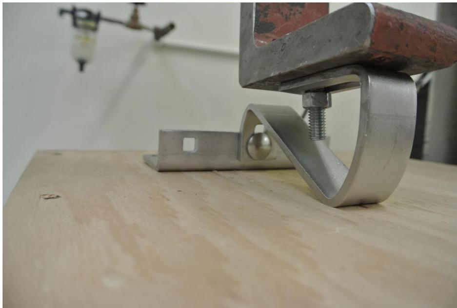
Figure 1b. Typical Failure Mode
