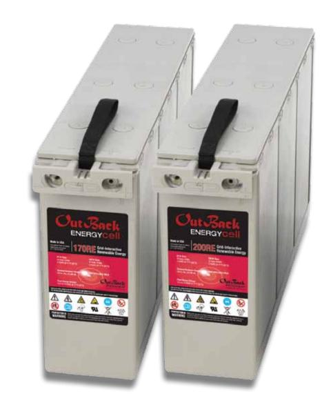
The EnergyCell RE Valve Regulated Lead Acid (VRLA) battery is designed for high power density and renewable energy cycling applications. Absorbed Glass Matt (AGM) technology provides for efficient gas recombination of up to 99% and freedom from electrolyte maintenance. The EnergyCell RE also features low profile terminals with threaded copper alloy inserts providing reduced maintenance and increased safety.
