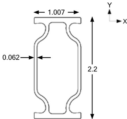
SOLARMOUNT-E Beam Height = 2.200"
